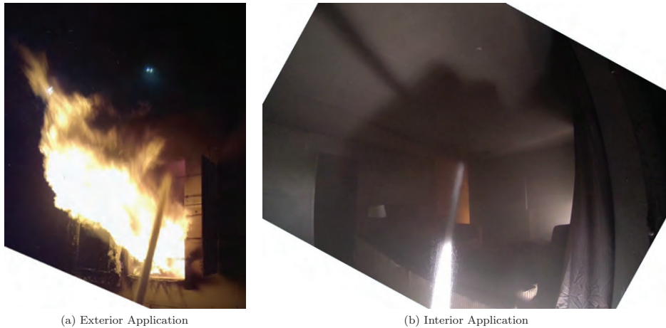
Figure 6.33: Water Application during Positive Pressure Attack
