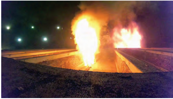
Figure 6.41: Fire From Simulated Balloon Frame Stud Cavity Prior to PPA
