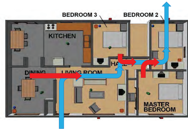
Figure 6.50: Air Entrainment From Connected Spaces
