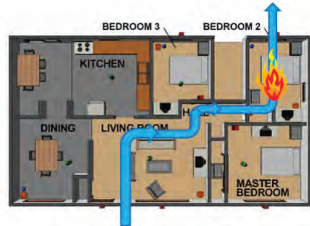
(e) Ventilation Configuration
