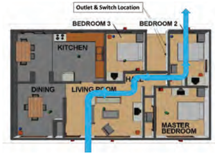
(b) Outlet and Switch Locations
