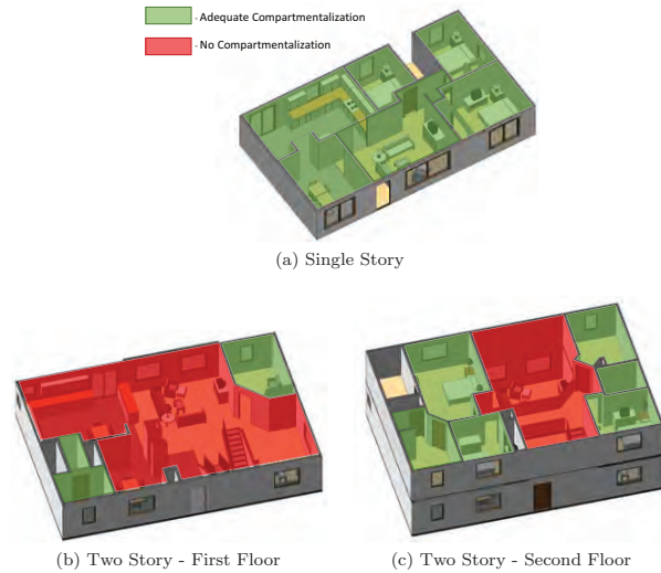
Figure 6.26: Understanding Compartmentalization of Structures
