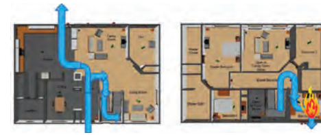
Figure 6.22: Two Story Structure Access from Side C
