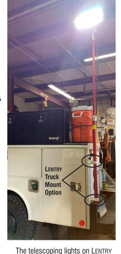
LIGHT SYSTEMS detach with the turn of a knob so they can be carried and stored separately from the rest of the unit. The Truck Mount option allows the lights to be easily stowed or used on the truck, as shown above with a V-Spec LED on an XT height pole. Photo courtesy of Connecticut Water Company, CT.
