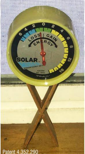
To use: place on a mount with the back of the Solar Miser flush with the window (shown at left) or mounted directly onto the window (shown below).
